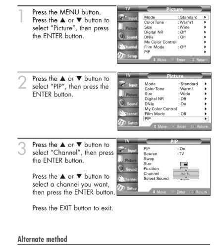
Press the CH $\land$  or CH $\checkmark$  button on the remote control to change channels of sub picture during PIP on.
